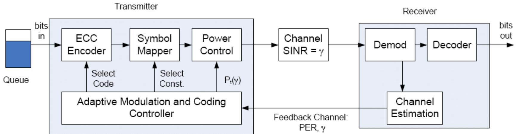
Figure 6.7: Adaptive Modulation and Coding Block Diagram.
